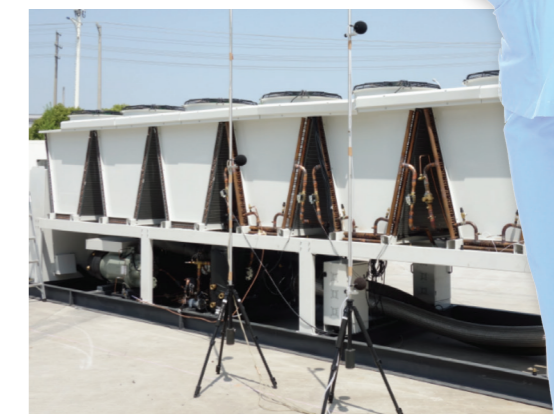
Sound power test confirmed RTAG complies with the requirements of ISO 3744 standard.
