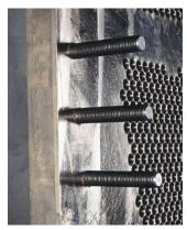
Available corrosion-resistant copper-nickel or titanium-clad tube sheets can be specified.
